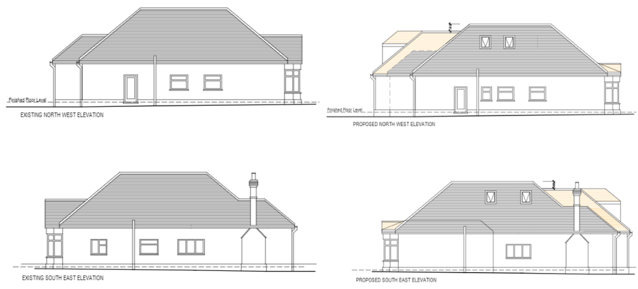
Figure 10 & 11 – Existing (left) and Proposed (right) side elevations
